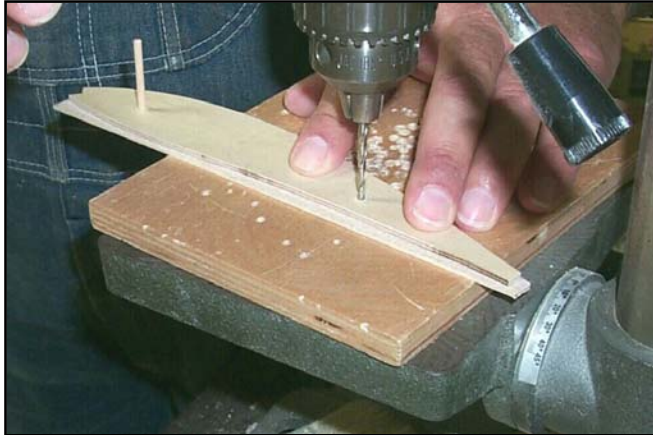
Figure 13 drilling holes in roughed out balsa ribs
