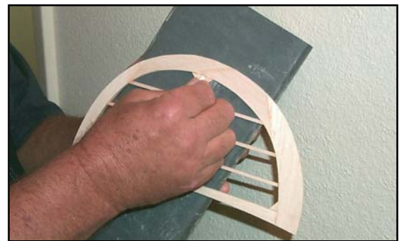
Figure 11 sanding rudder flat both sides
