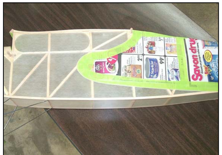
Figure 39 one side of fuselage masked as described with 3M Fine Line and 3M Scotch 233+ masking tape. Works great!
