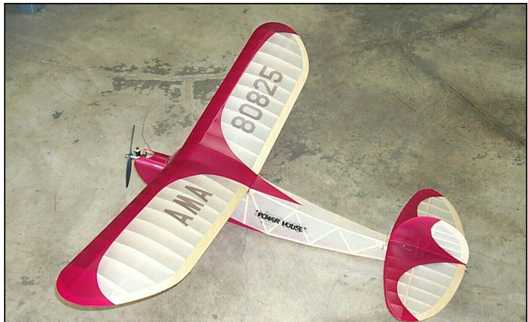
Figure 41 Masking is stripped after nitrate dried, ready for fuel proofing
