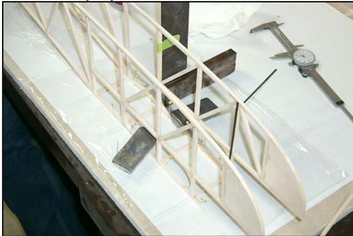
Figure 26 joining the two fuselage sides
