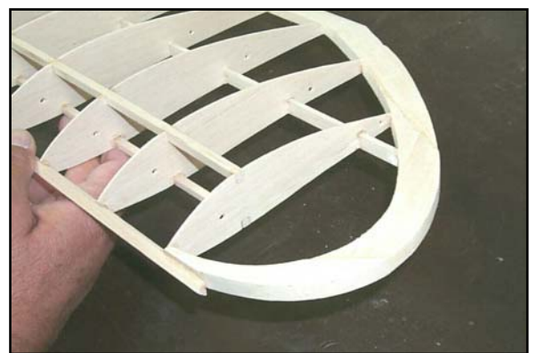
Figure 16 shows 3/8" balsa tips installed
