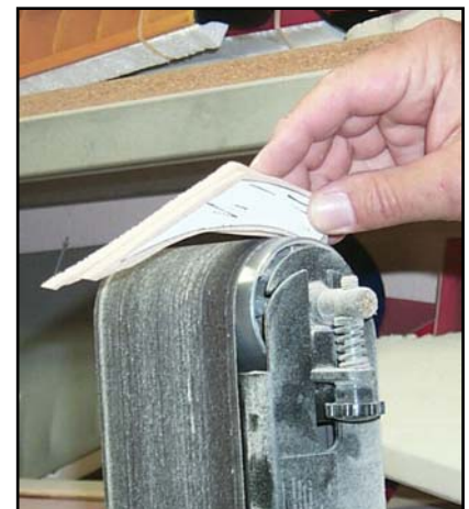
Figure 6 sanding inside radius
