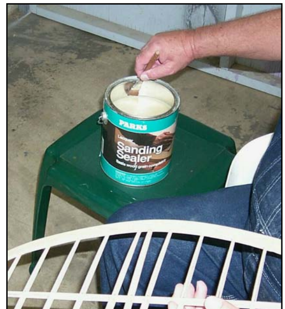
Figure 30 brushing on sanding sealer
