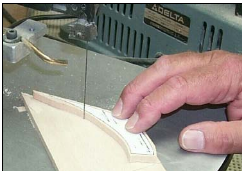
Figure 5 cutting a second stacked part
