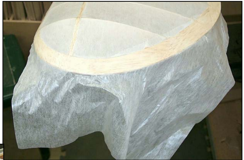
Figure 35 a completed wing tip shrunk and attached
