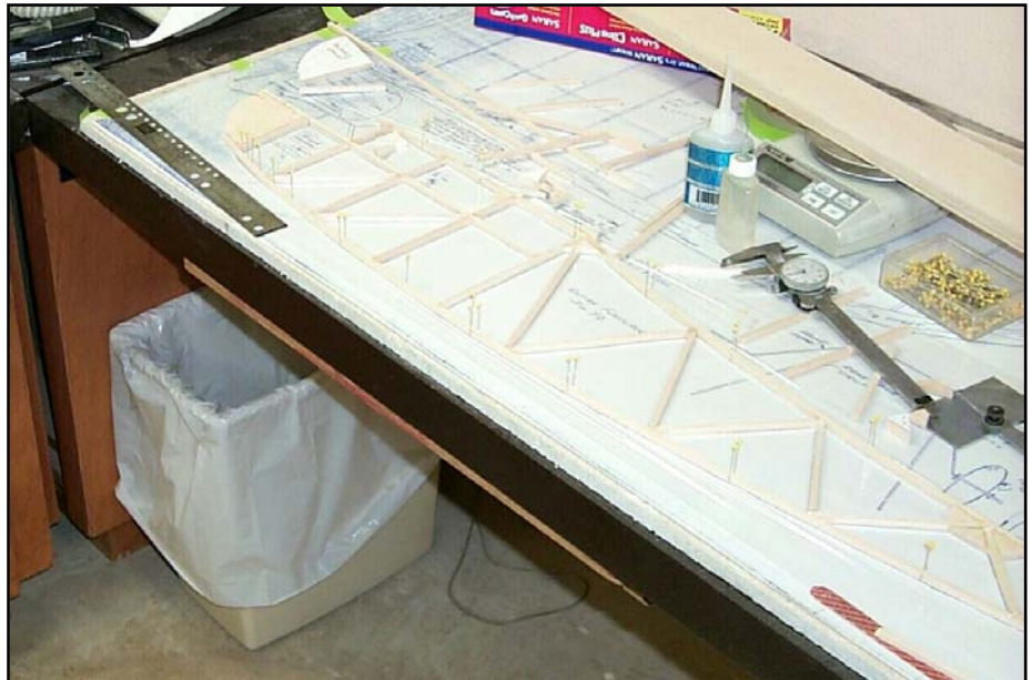
Figure 21 shows one fuselage side on plan, note calipers, scale & angle finder
