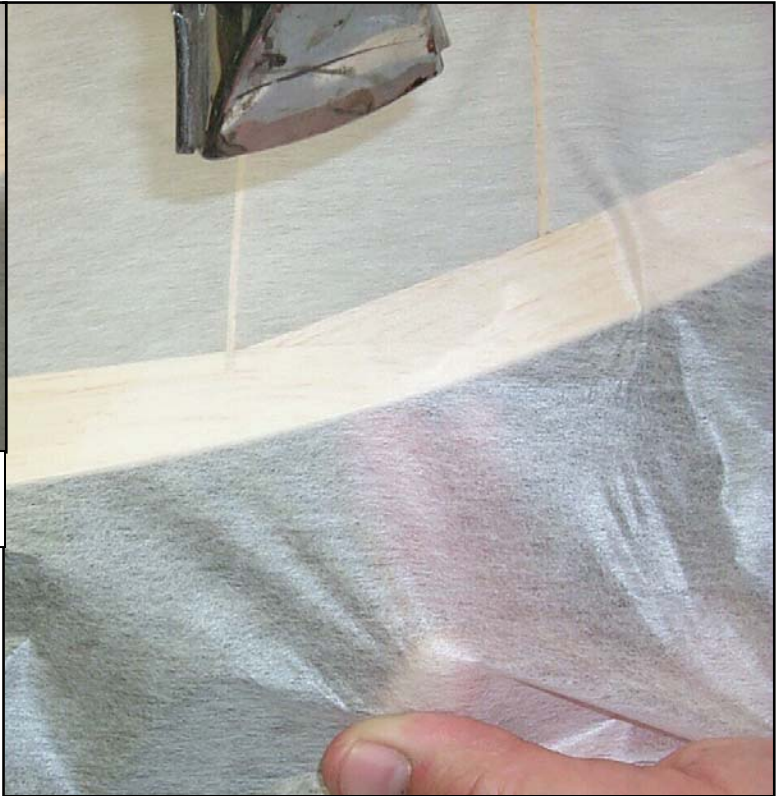
Figure 34 I use a MonoKote heat gun to shrink out wrinkles
