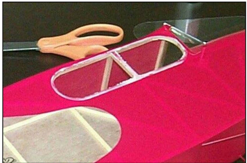
Figure 43 side window is set in place over a small bead of Formula 560 glue. Set in place to avoid smearing glue
