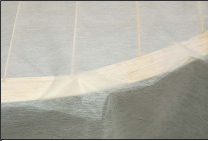
Figure 33 again shows wrinkle to be shrunk with heat
