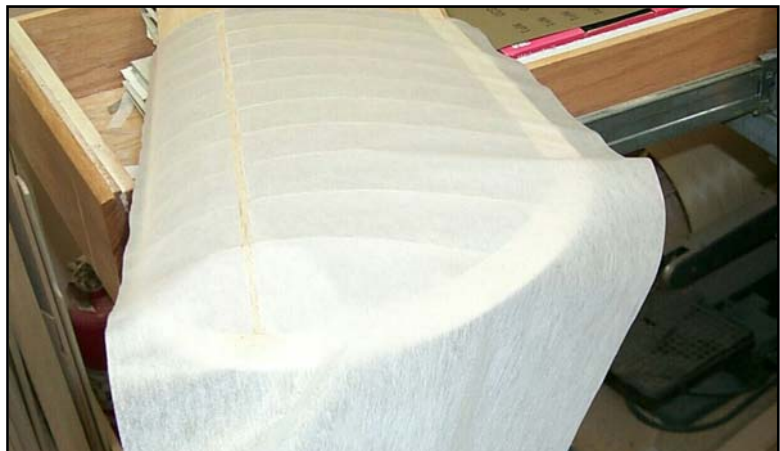
Figure 32 covering attached to spar with Acetone
