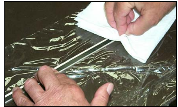
Figure 8 building a carbon laminated spar
