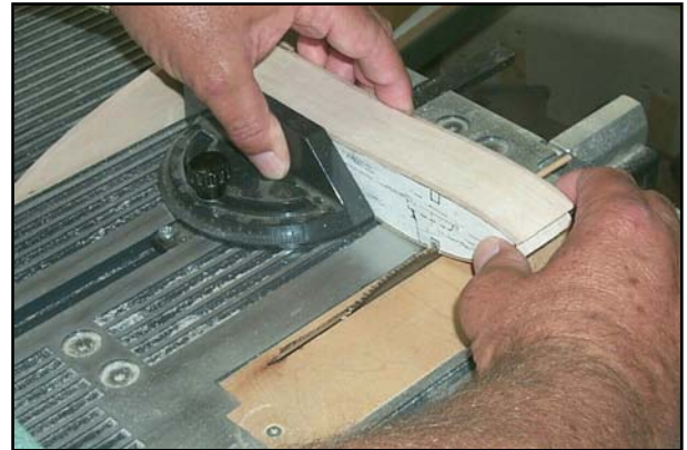
Figure 14 cutting notches for spars
