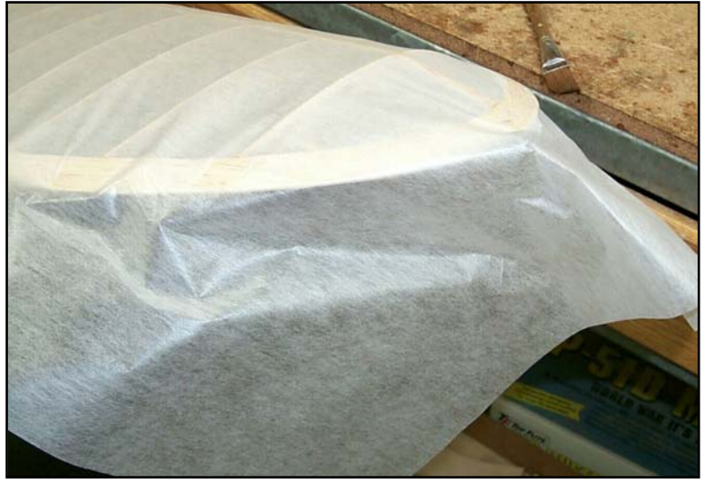
Figure 31 covering on wing tip, note wrinkles
